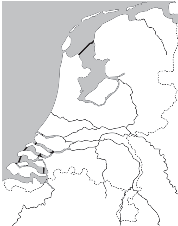
Fig. 3. Deep-sea inlets and large inland saltwater lakes such as the Zuider Zee have been cut off from the sea, reducing the country's coastline by hundreds of kilometres
