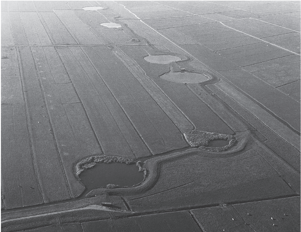
Fig. 2. Along the dike deep pools have been scoured out by water swirling through breaches which still can be seen in the landscape. Zomerdijk. Photo: Henk Bol. Province Utrecht
