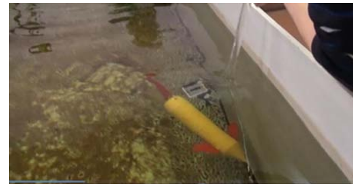
Autonomous remotely controlled robot-fish (RTU)
