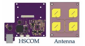
Nanosatellite high-speed communication subsystem (HSCOM)
