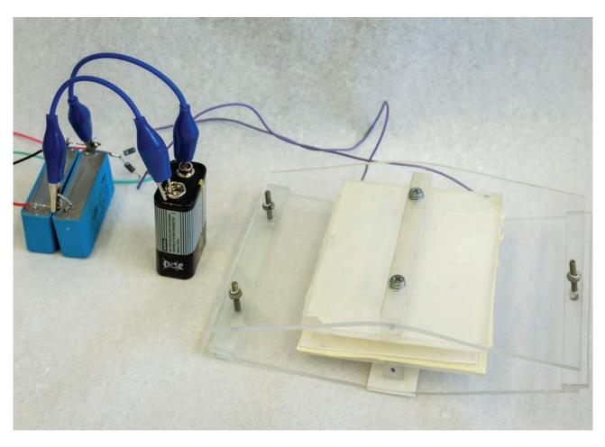
Triboelectric nanogenerator device using electrically polarized ferroelectric contact layers
