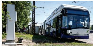
Test refuelling of hydrogen FC range extended trolleybus in Rīga
