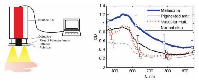
*Fig. 2.* Multispectral imaging setup and average OD spectra from melanoma, benign pigmented lesions, vascular lesions and normal skin [6]
